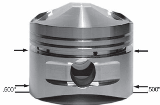
MEASURE CLEARANCED PISTONS HERE
