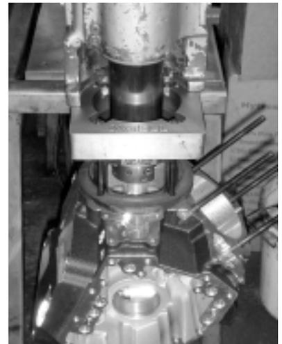
After completing this operation, install the case assembly into a mill or boring bar. Bore out the spigot holes to accept the new cylinders. All cases will need to be bored to 1.500" deep. Be careful not to exceed this distance, as you stand a great chance of cutting into vital oil passages.
