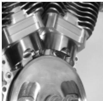
Now, slide the cylinders down until they are seated. Check the deck clearances at TDC and make changes to your squish accordingly.
